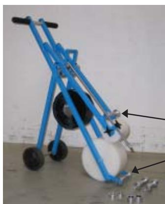
The spacers must fit the width of the roll.
