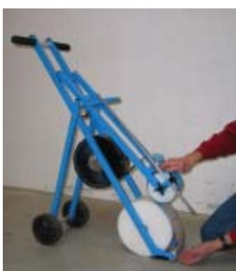
The DuraStripe must be tight around the steer roll. Lock the spring arm.
