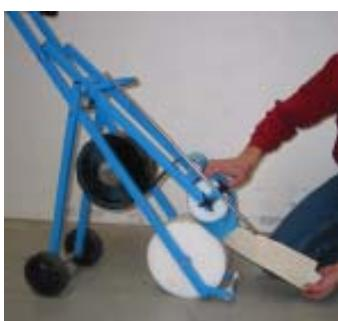
The foil is wrapped around the top wheel. Tip: Fasten the foil with some tape. Separate the foil from the tape.
